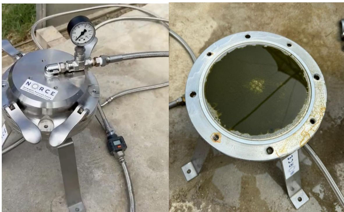
Figure 5 – Microplastics Sampling device (left) and clogged filter after 5 litres filtration at FURG IMTA, Brasil
