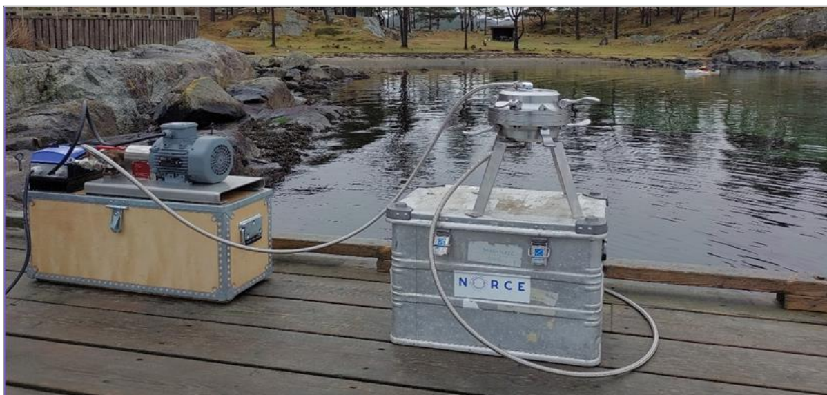
Figure 4 – Large Volumes Microplastics Sampling device engineered by NORCE for ASTRAL project. (Credit: Alessio Gomiero).
